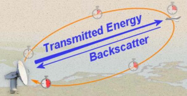
Reflection of electromagnetic waves
