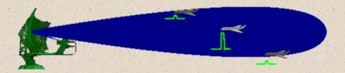
The antennas of most radar systems are designed to radiate energy in a onedirectional lobe or beam that can be moved in bearing simply by moving the antenna. The point of maximum echo, determined by the detection circuitry or visually by the operator, is when the beam points direct at the target. Weaponscontrol and guidance radar systems are positioned to the point of maximum signal return and maintained at that position either manually or by automatic tracking circuits.
